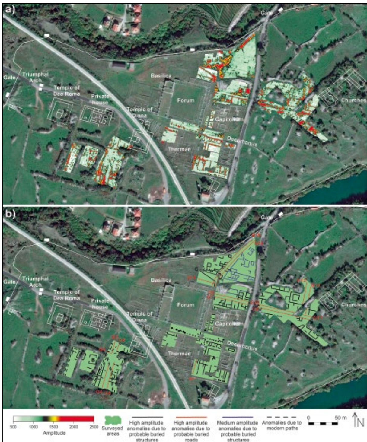
Plate 4 – GPR results: time slice relative to the time window 14-18 ns (about 0,7-1,4 m in depth), overlapped on the satellite image of Google Earth™ (a) and identification of anomalies (b).
