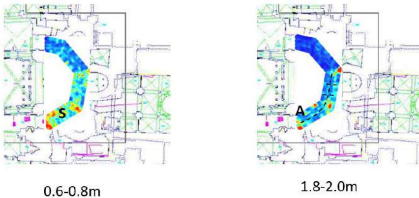
Fig. 89: Area OO: depth slices overlapped to the planimetry
