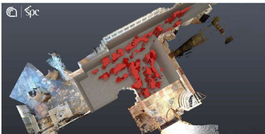
Fig. 50: the whole Area: virtual-excavation: 1.6-1.8m depth
