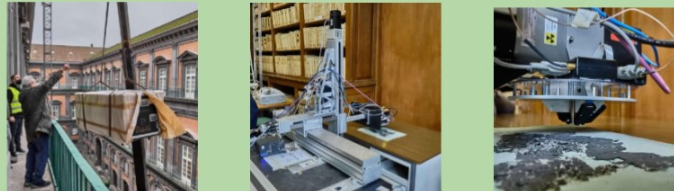
Macro-X-Ray Fluorescence Imaging Instrument (CNR-ISPC, Catania) being lifted (left) and in operation (middle); detail of the same (right)
