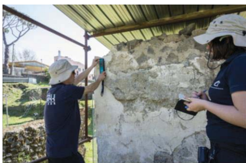
Fig. 6. Micro-resistivity data acquisition
