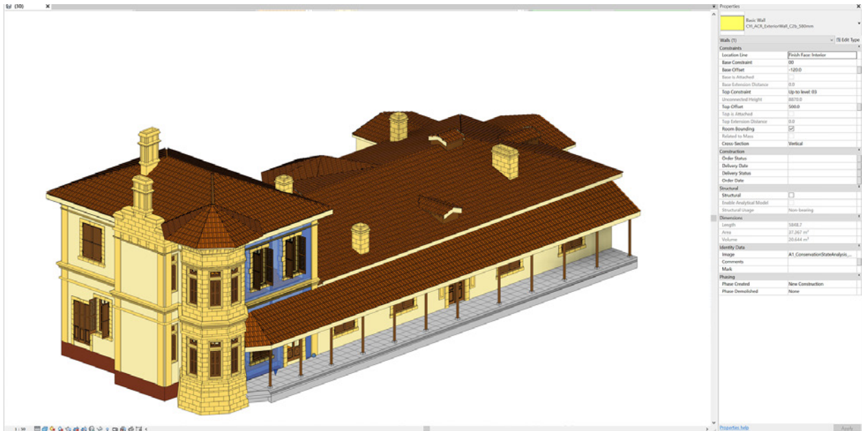
Fig. 9. Object selected to view its properties in the BIM model of the Cypriot pilot building.
