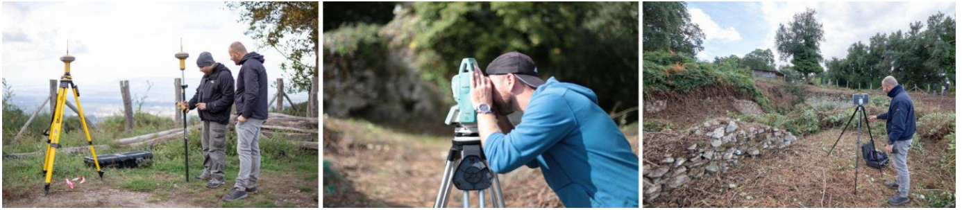
Figure 8. From left to right: topographic survey of GCPs using a differential GNSS; measurement of photogrammetric targets placed on archaeological structures with total station; 3D survey of a cistern with the laser scanner.
