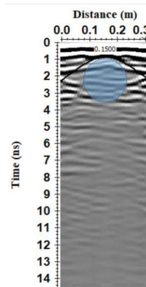
Fig. 3. GPR radar section with the diffraction curve analysis
