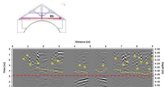
Fig. 7. The processed radar section
