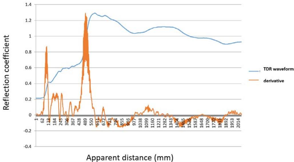
Fig. 1. The location of geophysical surveys TDR waveform (blue curve) and corresponding first derivative (orange curve) obtained for the wet maple
