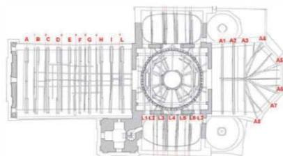
Fig. 6. The roof planimetry: the red letters refer to the position of the wooden structures
